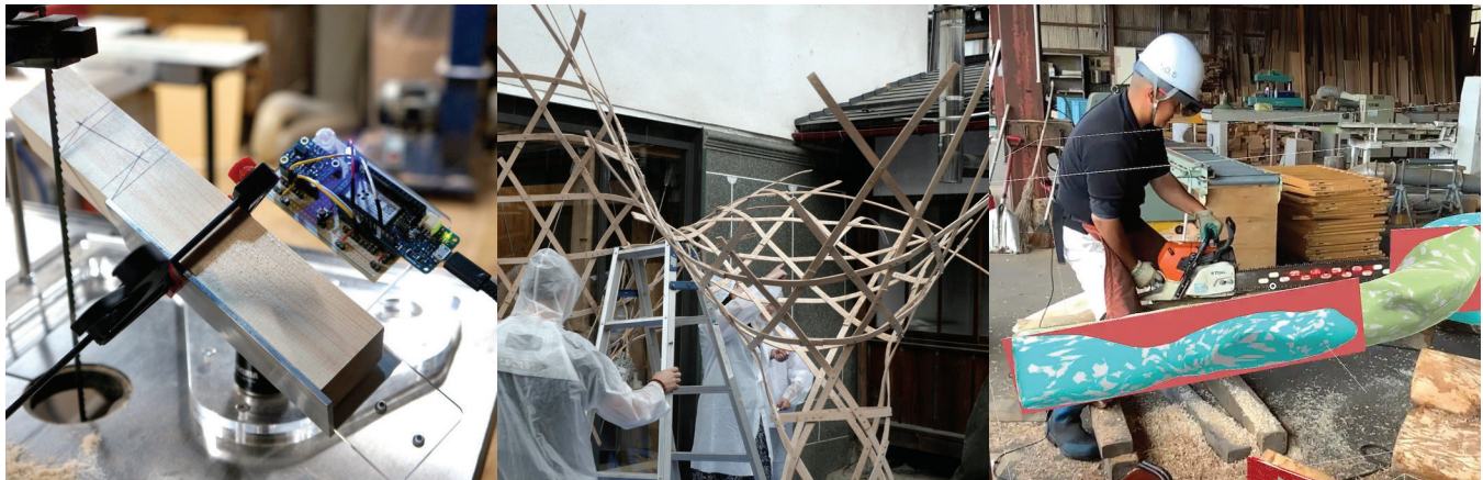
Figure 2. wood cutting jig with sensor (2018 workshop), compressed timber weaving (2019 workshop), Torinosu fabrication (2020). Bruscia, Hidakuma.
